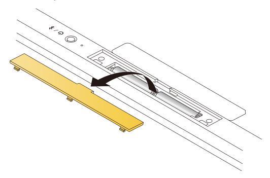
2) Remove the batteries.
