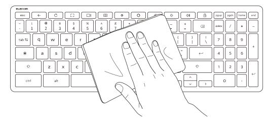
4) With the spacebar at the bottom, tilt the keyboard (30 to 45 degrees), leave it for at least 24 hours, and let dry.
