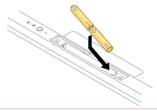
Do not use batteries of different types or use a mixture of old and new batteries. The batteries may leak fluid, causing a malfunction.
