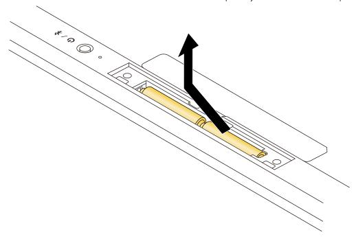
3) Insert the batteries according to the direction indicated in the battery storage compartment.
