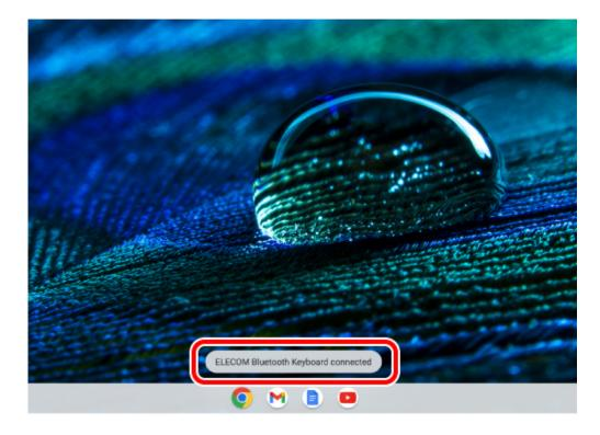
Click "Bluetooth" following the same procedure as in step 2. If "ELECOM Bluetooth Keyboard" is displayed under "Currently connected", pairing is complete.
